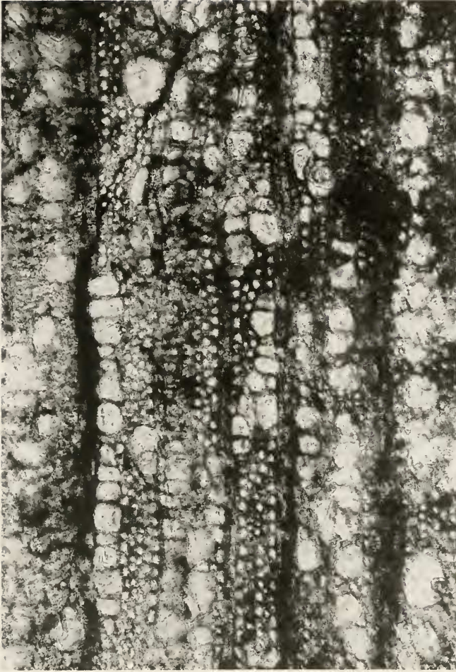
Fig. 3. Cross section. Late wood pores in long radial multiples, fibres in radial rows forming solid tracts between rays and vessels. x 130.
